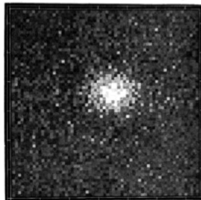
Fig. 21. Differential speckle image of \alpha Ori (Betelgeuse) showing a significant resolved structure at diameters to 100 msec of arc. The photon and atmospheric statistics in this preliminary sample of \sim 1000 frames of data limit this result to an effective signal maximum to a rms background noise ratio of \sim 10:1 . Scale: 5 msec of arc/pixel (compare with Fig. 20).
